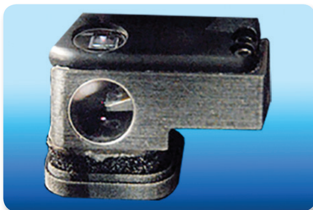
Figure 2. Environmental Control and Heater for nanoIR2 and 3 series products.
