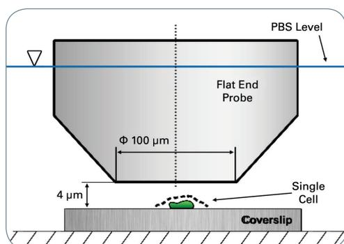
Figure 1. Schematic of a single cell compression test.
