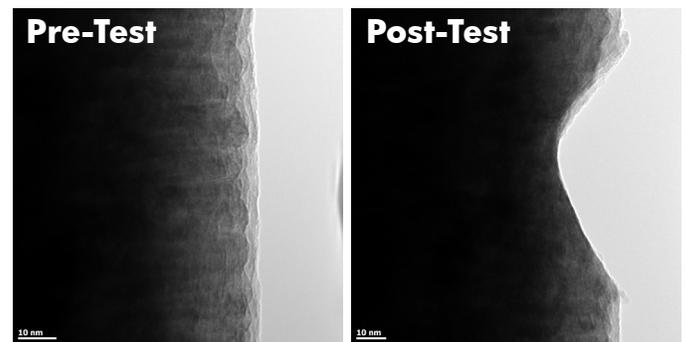
Figure 4: A load-depth plot from the in-situ testing and TEM micrographs of the film stack before and after deformation.
