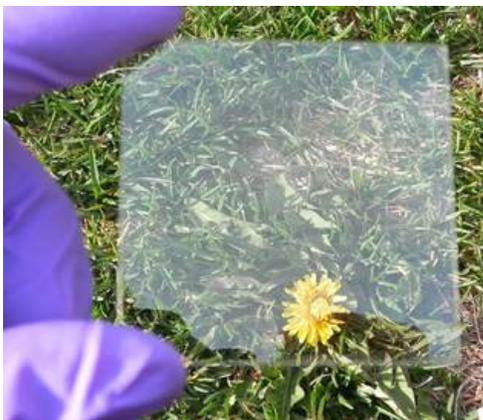
Figure 1: Combinatorial library, spread of composition of indium-zinc-tin-oxide (In-Zn-Sn-O) thin film by co-sputtering of indium oxide, zinc oxide, and tin oxide targets on 2”x2” glass substrate.
