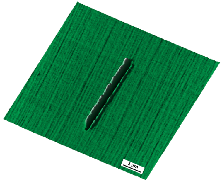
Figure 1. 8 µm SPM image of residual wear track left after reciprocating wear test on DLC film.
