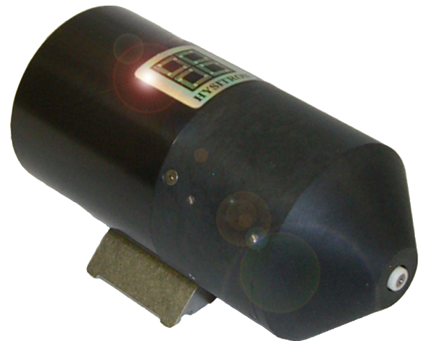
Figure 1. Photograph of MultiRange NanoProbe transducer head.
